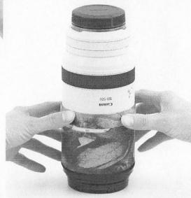
8.将⑧号炮衣套在功能环上,安装完成 Slide the lens cover ⑧ from the rear end of the lens.
